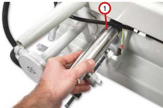
Fig. 8.1.2.5: Remove UV disinfection housing
