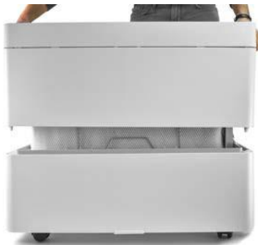
Fig. 6.3.1.1: Removing the upper part of the housing
