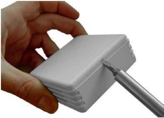
Fig. 5.6.3: Opening the cover
