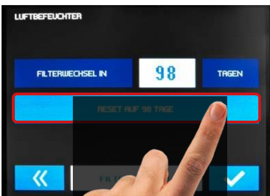
Fig. 6.3.2.7: Reset filter change indicator
