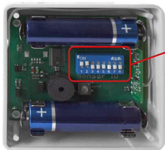
Fig. 5.6.1: Interior view of radio humidity transmitter
