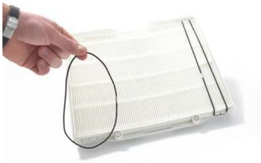
Fig. 6.3.2.2.2: Loosening the retainer
