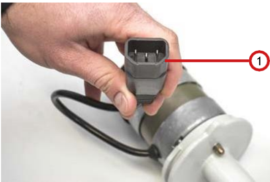
Fig. 7.4.1.7: Loosening the plug connection
