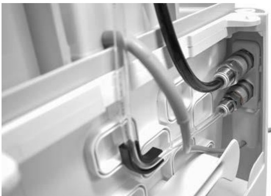
Fig. 6.3.4.4: Connection of power cable, AWS & flushing device
