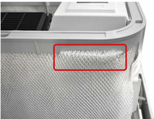
Fig. 6.3.2.5: Incorrect fit of the filter
