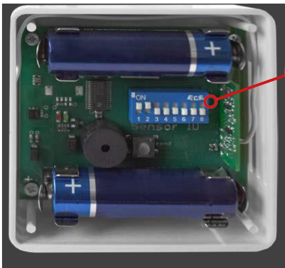
Fig. 5.6.4: Coding the radio humidity transmitter
