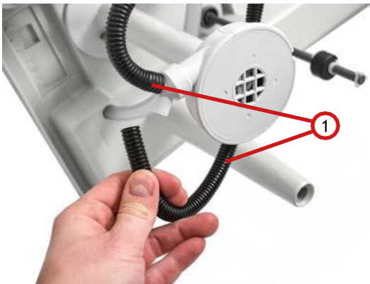
Fig. 6.3.4.4: Pulling off the pump hoses
